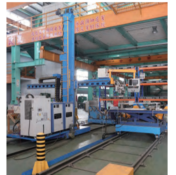
Welding Cross Arm
